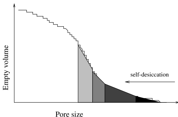
Fig. 2. Hypothetical pore size distribution for cement-based materials indicating that as more empty porosity is created due to self-desiccation, smaller and smaller pores are being emptied, in analogy to the filling of pores by mercury during an intrusion experiment.
