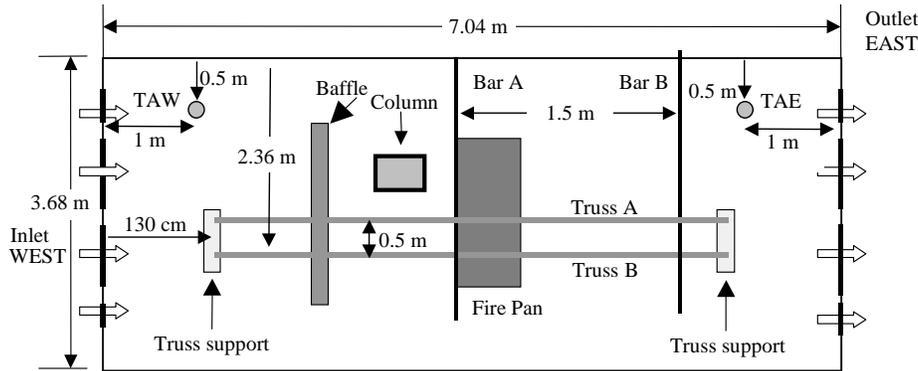
Fig. 1. Plan view of the experimental configuration.
