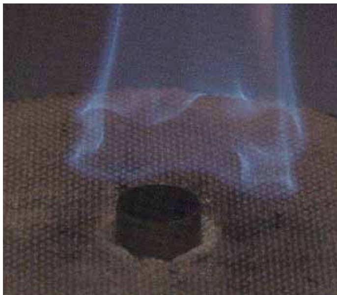
Figure 26. A time-resolved photograph taken by a digital camera shows the oscillating propane flame burning in air diluted with nitrogen. The complex azimuthal structure of the flame base, which has a much larger area than the burner tube, is clear.
