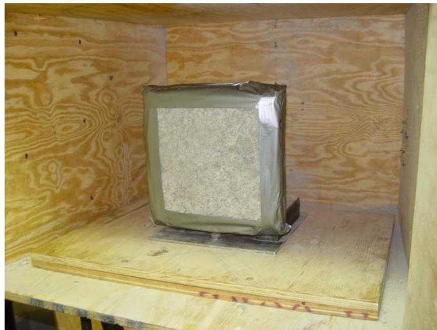
**Figure C-8. Photograph showing the edges of the SFRM duct taped to the steel plate before the ballistic tests at 0 degree.**
