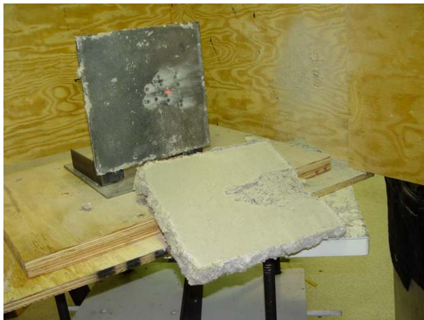
**Figure C-6. Photograph showing damage to the SFRM after a ballistic impact at 40 degree. The SFRM layer completely separated from the steel plate.**
