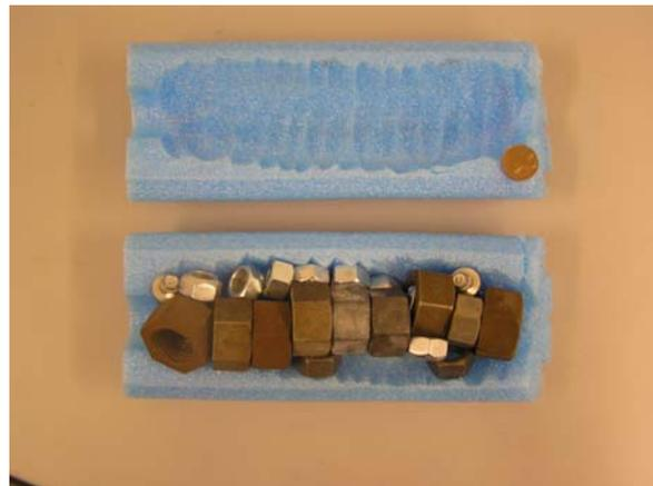
**Figure C-2. Typical shot shells used in the large universal receiver. A penny is also shown for comparison.**
