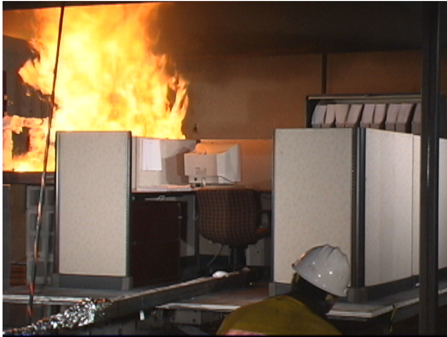
Figure 3–7a. 2 MW igniter flame at time zero.
