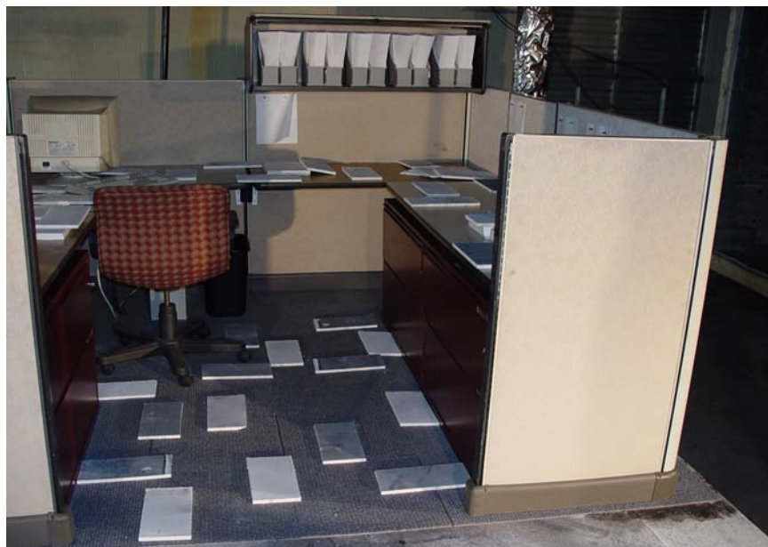
Figure 2–4. View from the south of the generic work station with calcium silicate “tiles” in place on exposed, upward facing surfaces (floor, desk, chair seat).
