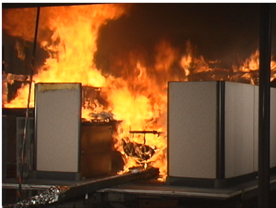
Figure 3-7d. Collapsing chair fire near its peak at 512 s.
