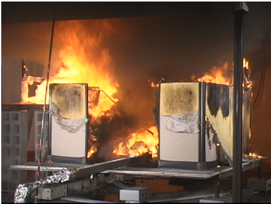
Figure 3-7f. Fire well past peak, with rear desk surfaces collapsed, at 965 s.
