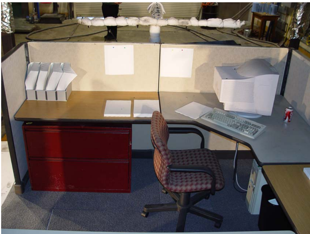
Figure 2–2. View from above of the west side of the generic workstation. The horizontal insulated pipe above the west wall is the feed line to the four nozzles of the spray igniter.
