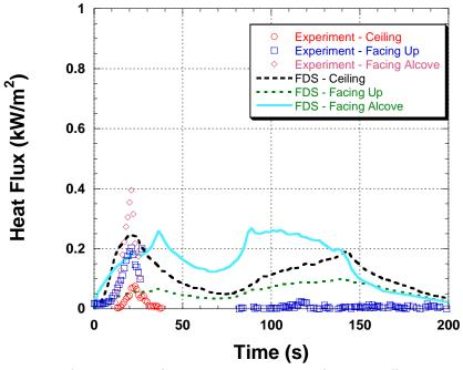
Figure 5-32. Heat flux comparison between the sprinklered fire experiment and the FDS simulation at Station D.
