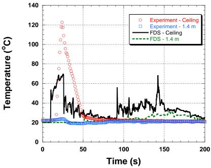
Figure 5-30. Temperature comparison between the sprinklered fire experiment and the FDS simulation at Station D.
