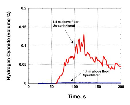
Figure 4-34. Hydrogen Cyanide Volume Fraction vs Time for Unsprinklered and Sprinklered Mockup Test. Gas Sampling probe positioned on Main Floor (Location C) at 1.4 m (4.5 ft) above floor.
