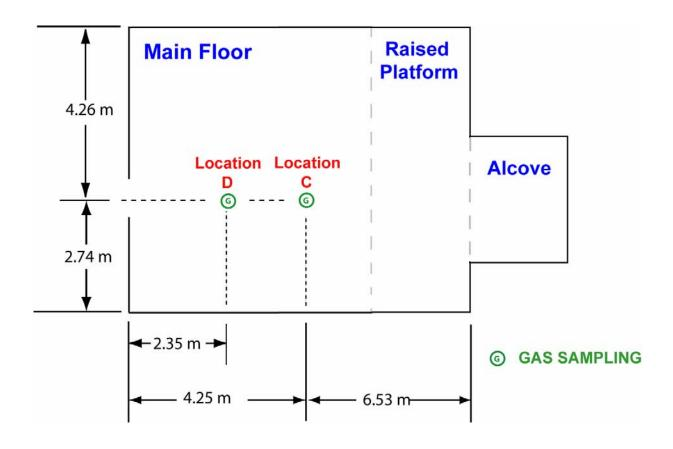
Figure 4-29. Schematic floor plan with gas sampling locations.
