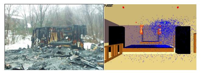
Remains of the platform area after the fire (left) and an image from the simulation of The Station fire had sprinklers been installed (right)
