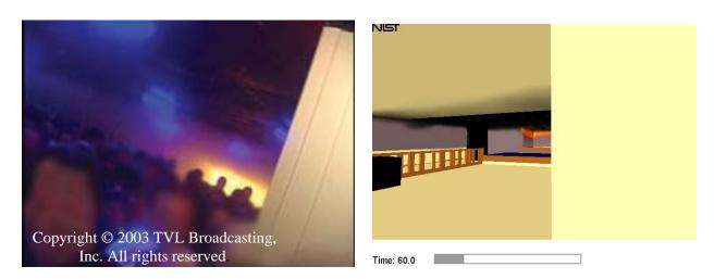
Figure 5-46. Smoke beginning to roll across ceiling (video 53 seconds, simulation 60 seconds)
