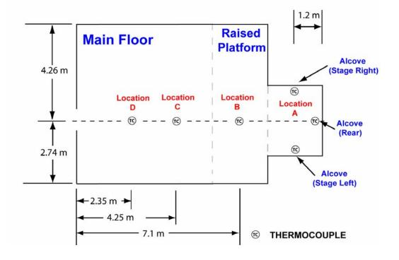
Figure 4-21. Schematic floor plan with thermocouple positions.
