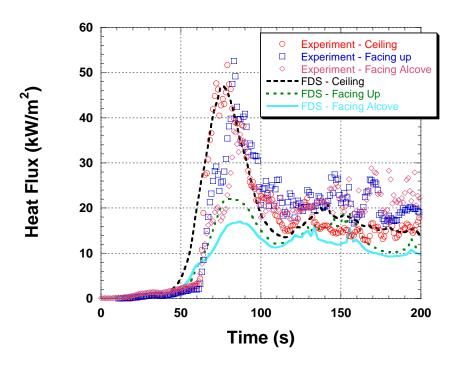
Figure 5-15. Heat flux comparison between the un-sprinklered fire experiment and the FDS simulation at Station C
