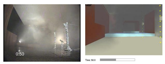
Figure 5-25. Fire suppression continues in both the experiment and the simulation, t = 50 seconds after ignition.
