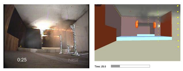
Figure 5-22. Initial sprinkler operating, t = 25 seconds after ignition.
