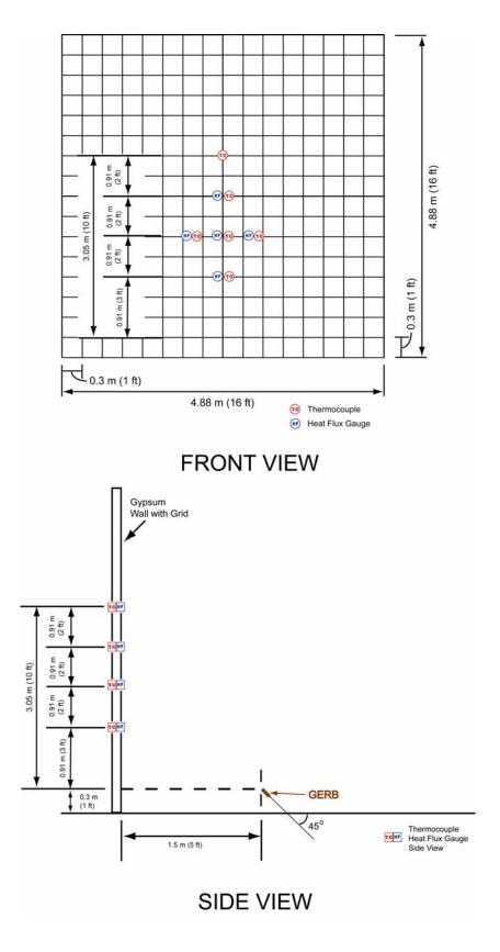
Figure 4-12. Instrumentation Diagram for a Single Gerb at 45 degrees and in a Plane Perpendicular to Wall.
