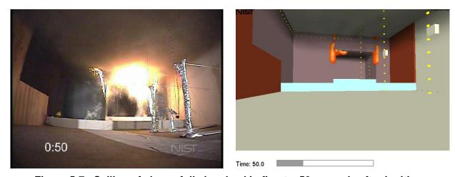
Figure 5-7. Ceiling of alcove fully involved in fire, t = 50 seconds after ignition.
