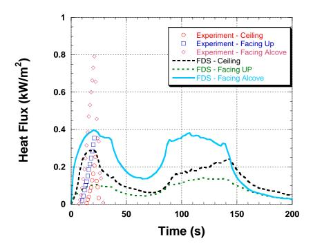
Figure 5-31. Heat flux comparison between the sprinklered fire experiment and the FDS simulation at Station C.
