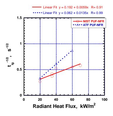
Figure 4-2b. Time to sustained ignition versus external heat flux for different polyurethane foams tested at NIST and ATF.
