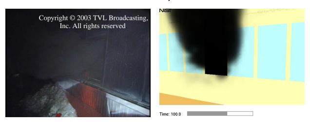
Figure 5-47. Smoke billowing outside from broken sunroom window (100 seconds)
