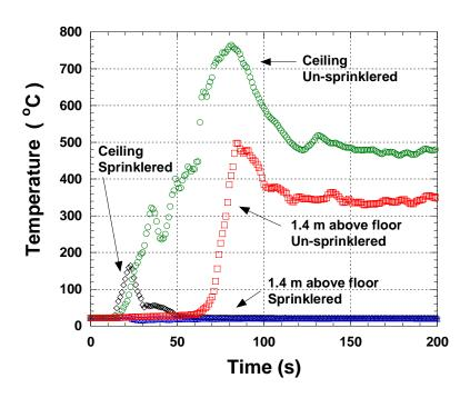
Figure 4-28a. Temperatures versus Time for Unsprinklered and Sprinklered Mockup Test. Thermocouples positioned on Main Floor (Location C) at ceiling and 1.4 m (4.5 ft) above floor.
