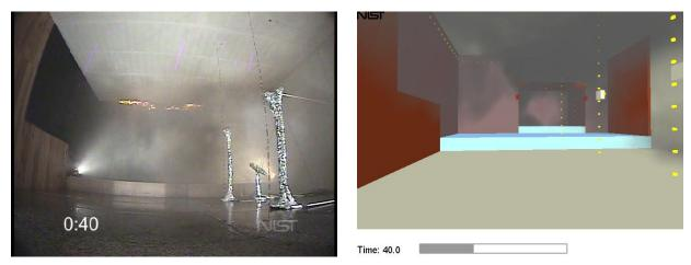
Figure 5-24. Suppression with three sprinklers operating in each case, t = 40 seconds after ignition.
