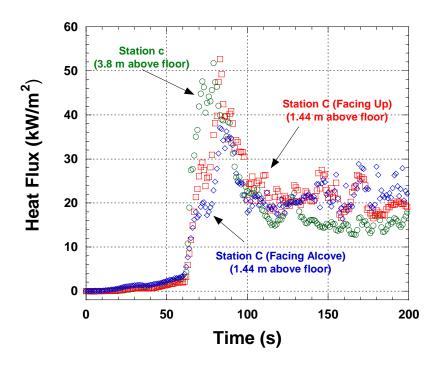
Figure 4- 37. Heat Fluxes versus time for unsprinklered mockup test. Radiometer positioned flush with ceiling (3.8 m above floor); heat flux gauges facing up (1.44 m above floor), and facing alcove (1.44 m above floor) at sampling location C.
