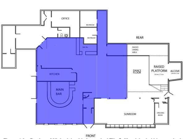
Figure 4-3. Portion of Nightclub with Acoustical Tile Ceiling (shaded blue section).
