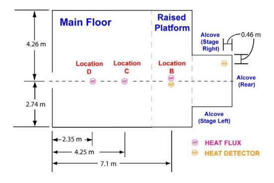
Figure 4-36. Schematic floor plan with heat flux and heat detector locations.
