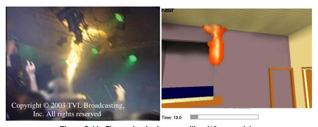
Figure 5-44. Flames impinging on ceiling (19 seconds)
