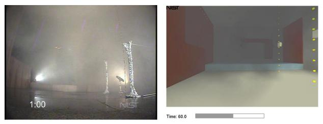
Figure 5-26. Fire controlled in both cases, t = 60 seconds after ignition.
