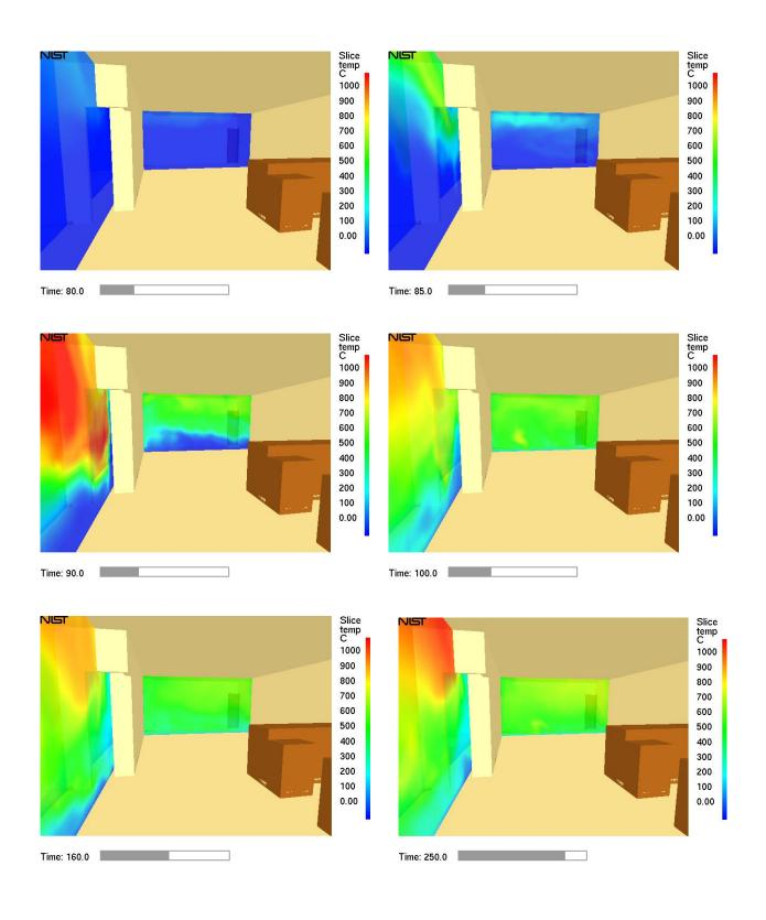
Figure 5-60. Temperature profiles in the dart room, 80 seconds to 250 seconds
