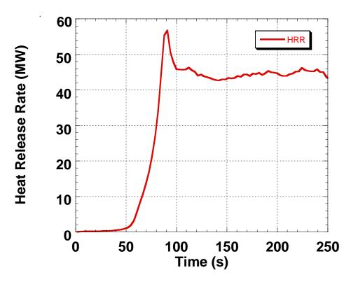
Figure 5-42. Total Heat Released in Building Fire Simulation as a Function of Time
