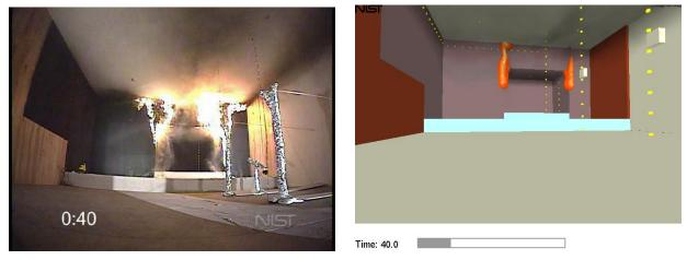
Figure 5-6. Flames continue to spread into alcove, t = 40 seconds after ignition.
