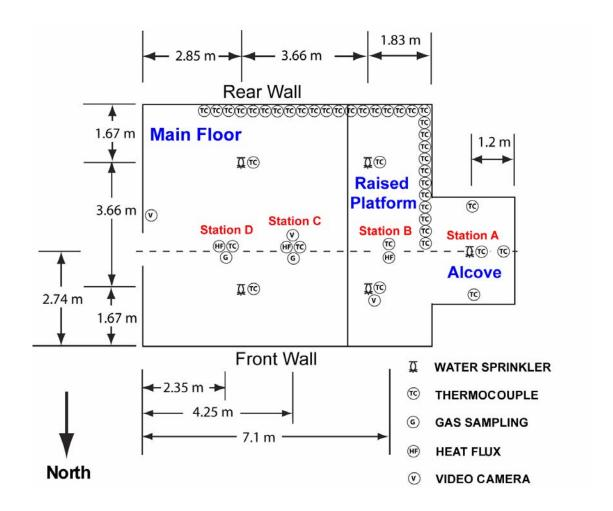
Figure 4-19. Schematic floor plan with instrumentation positions.
