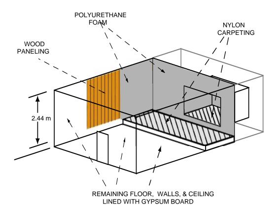
Figure 4-18. Floor plan showing the test area and the fuel locations.
