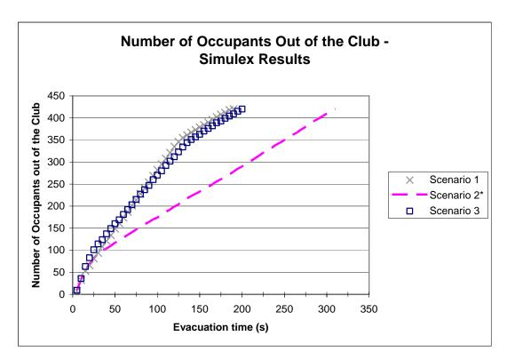
Figure 6-17. Cumulative plot of evacuation from building for different scenarios calculated from Simulex [37, 38]. (Note that a non-zero pre-movement time would shift the curves to right.)
