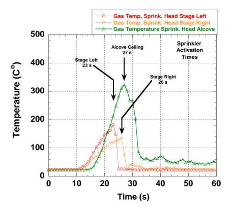
Figure 4- 42. Temperature versus Time for Sprinkler Thermocouples.
