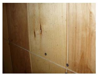
Figure 4-14b. Damage to wood panel following impingement by sparks from gerb. Lip on panel surface can be seen as line below mounting screws.
