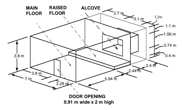
Figure 4-17. Isometric view of the test compartment.
