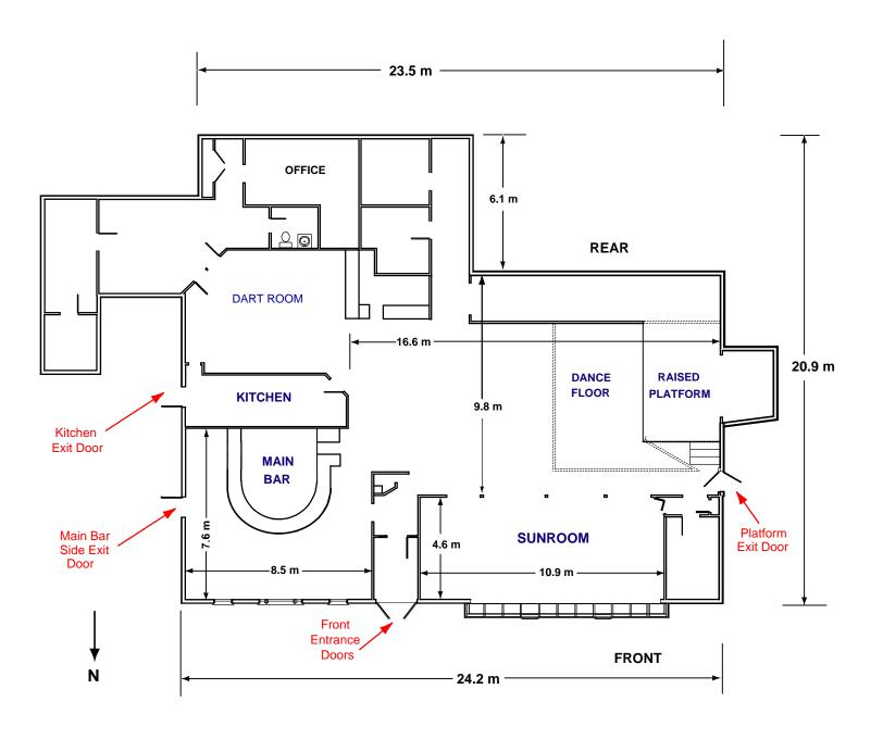
Figure 1-5. Plan view of The Station showing different rooms and exits.
