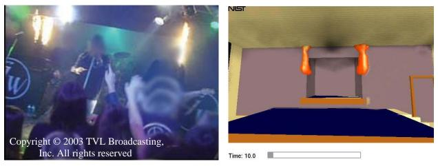
Figure 5-43. Initial growth of fire on foam at corner of the alcove (10 seconds)
