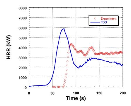
Figure 5-12. Power generated in experiment as measured outside of doorway, compared to FDS simulation of heat release rate from fire within compartment.
