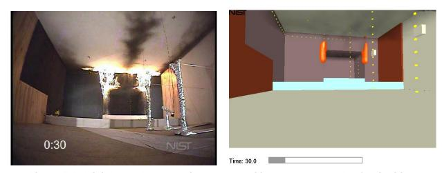
Figure 5-5. Visible smoke spreading across ceiling, t = 30 seconds after ignition.
