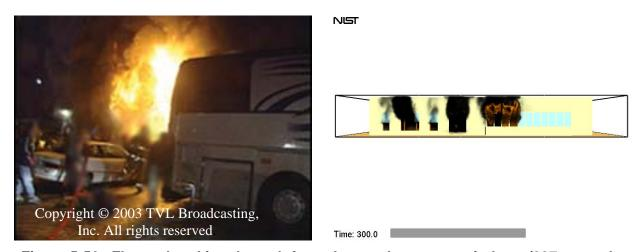
Figure 5-52. Flames breaking through front door and sunroom windows (337 seconds video, 300 seconds simulation)
