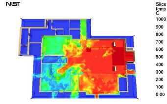
Temperatures 1.5 m (5 ft) above floor 90 seconds after ignition, calculated from computer simulation of full-scale nightclub fire.
