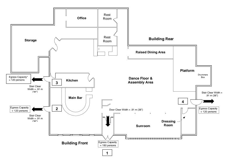
Figure 7-5. Station Nightclub Egress Capacity (\*Note that model codes exclude exiting through a kitchen when calculating occupancy limit.)
