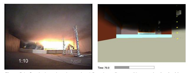
Figure 5-9. Smoke layer has dropped to 1.5 m above floor, t = 70 seconds after ignition.
