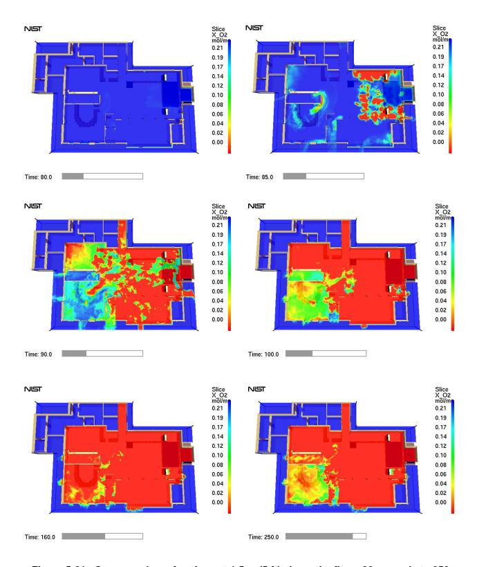
Figure 5-61. Oxygen volume fractions at 1.5 m (5 ft) above the floor, 80 seconds to 250 seconds
