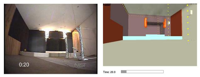
Figure 5-4. Flames impinging on ceiling, t = 20 seconds after ignition.
