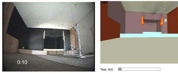
Figure 5-3. Flames spreading toward ceiling, t = 10 seconds after ignition.
