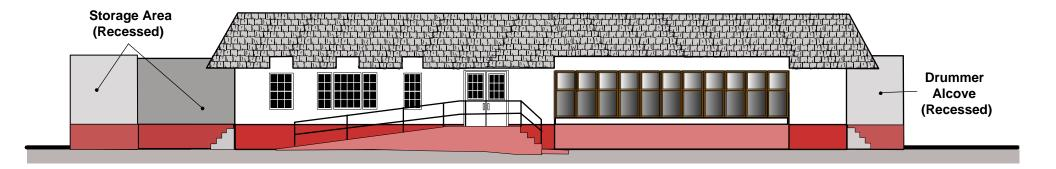
Figure 1-3. Sketch of the north side of The Station nightclub locating the main entrance, front stairway/ramp, windows in the main bar area (left), sunroom/pool room (right), and exit stairs from the east and west sides
