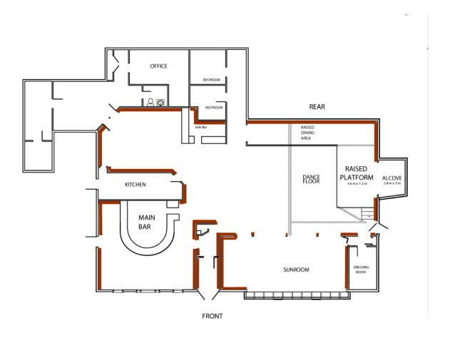
Figure 4-4. Portion of Nightclub with Wood Paneling (brown shaded sections).
