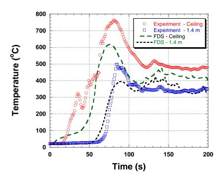
Figure 5-13. Temperature comparison between the un-sprinklered fire experiment and the FDS simulation at Station C.
