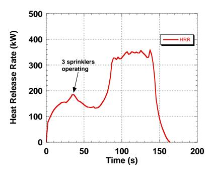
Figure 5-28. FDS predicted heat release rate for the sprinklered case.
