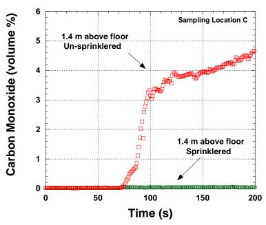
Figure 4-32. Carbon Monoxide Volume Fraction vs Time for Unsprinklered and Sprinklered Mockup Test. Gas Sampling probe positioned on Main Floor (Location C) at 1.4 m (4.5 ft) above floor.
