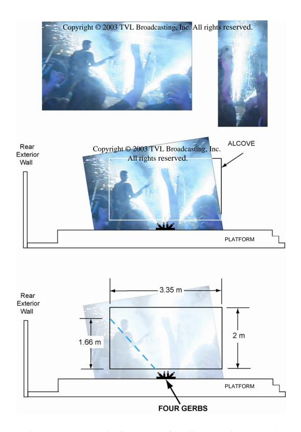
Figure 4-10. Pyrotechnics (15 x 15 gerbs) positioned on nightclub platform. Video image copyright © 2003 TVL Broadcasting, Inc. All rights reserved.
