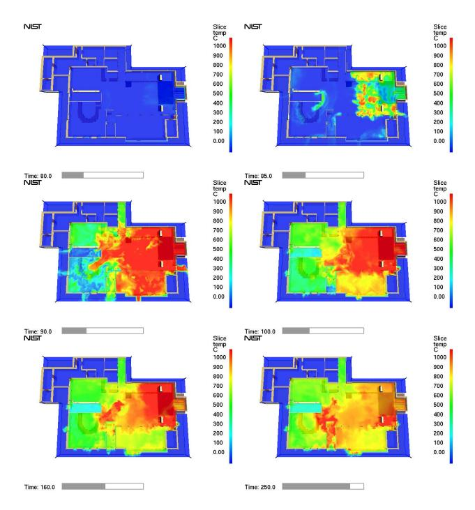
Figure 5-55. Temperatures at 1.5 m (5 ft) above the floor, 80 seconds to 250 seconds
