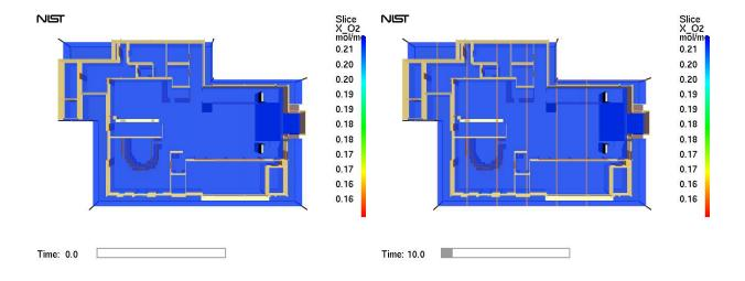
Figure 5.67a. Oxygen volume fractions at 1.5 m (5 ft) above the floor, 0 seconds and 10 seconds
