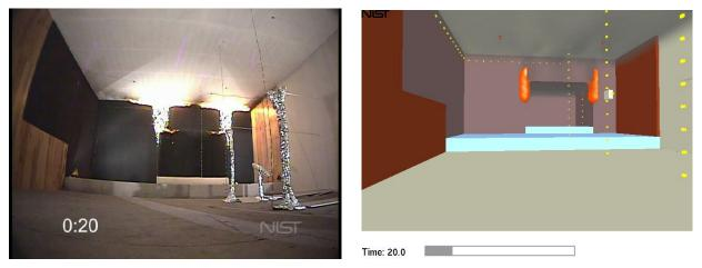
Figure 5-21. Flames impinging on ceiling, t = 20 seconds after ignition.
