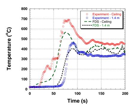
Figure 5-14. Temperature comparison between the un-sprinklered fire experiment and the FDS simulation at Station D.
