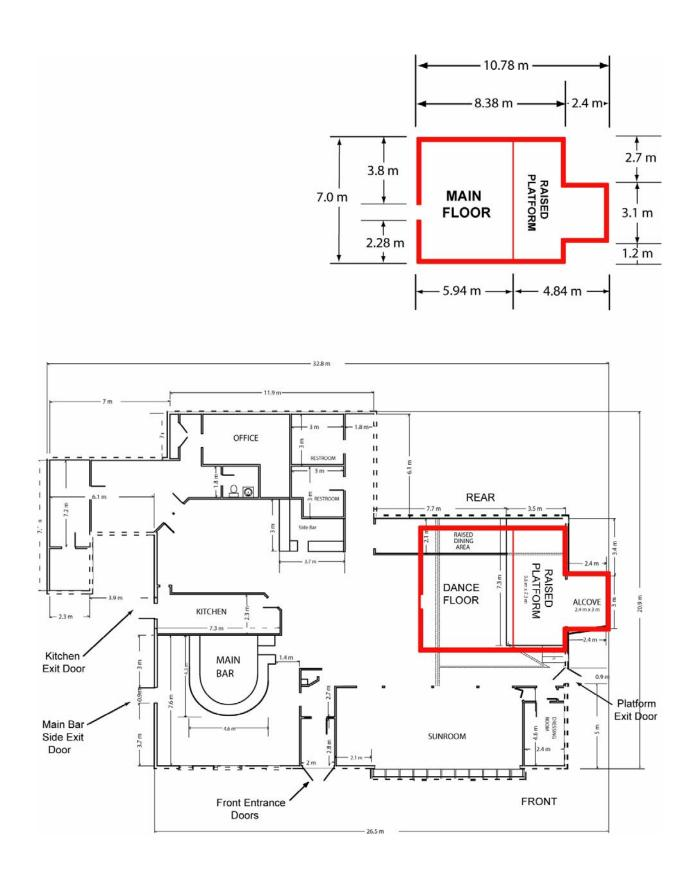
Figure 4-16. Real-Scale Mockup Floor Plan versus Station Nightclub Floor Plan.
