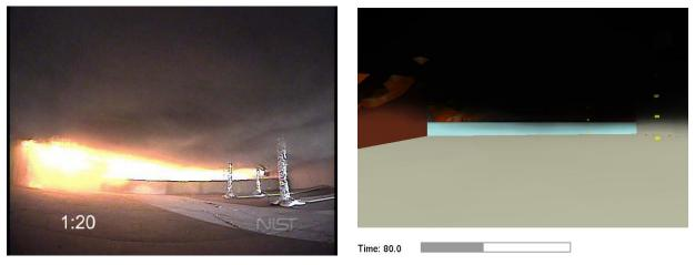
Figure 5-10. Fire continues to spread, t = 80 seconds after ignition.
