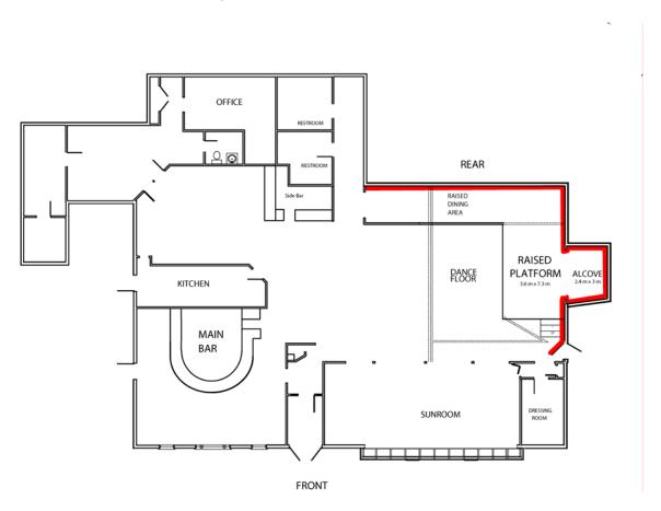
Figure 4-1. Portion of Nightclub with Polyurethane Foam Mounted on Wall (shaded red section).
