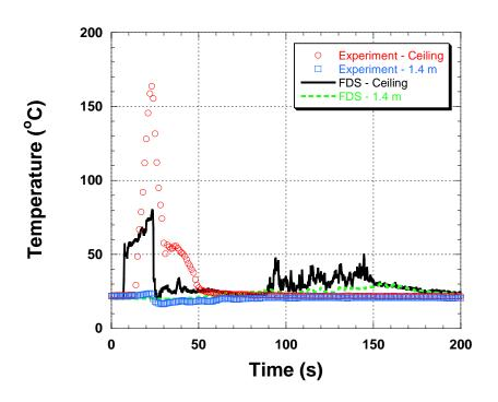
Figure 5-29. Temperature comparison between the sprinklered fire experiment and the FDS simulation at Station C.
