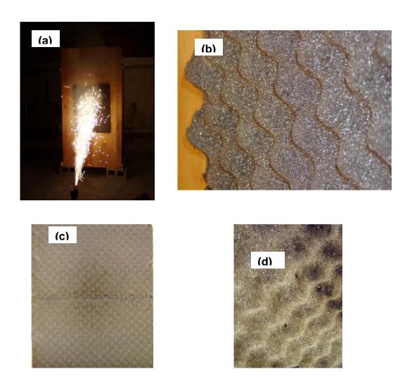
Figure 4-15. Gerb impinging fire retardant polyurethane foam (a); evidence of pitting (b); horizontal ledge at mid-plane to catch sparks, and evidence of scorching in second sample (c); and close-up of scorched area (d).
