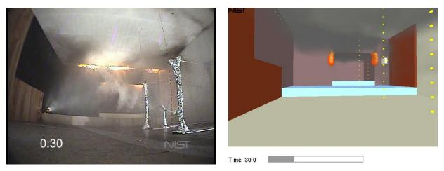
Figure 5-23. Third sprinkler operating in experiment, t = 30 seconds after ignition.
