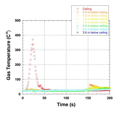
Figure 4-25. Temperatures versus Time for Sprinklered Mockup Test.
