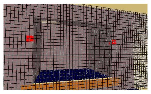
Figure 5-38. Numerical grid used for foam covered walls on platform. Red squares represent the points of ignition
