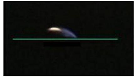
Fig. 3. Selected edge view image of flame over 0.2 mm thick PMMA (green line) in 21% O<sub>2</sub> at 5 cm/s with 6 s laser duration.  $t = 0.06$  s before laser termination.
