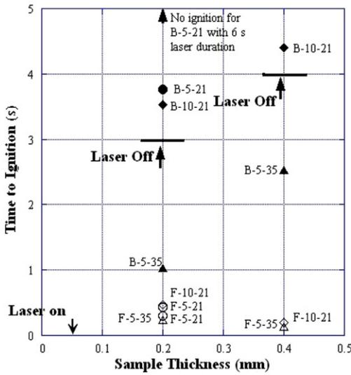
Fig. 1. Effects of sample thickness on ignition delay time of PMMA in microgravity. (F, frontside/B, backside)-flow velocity (cm/s)-O<sub>2</sub> (%).
