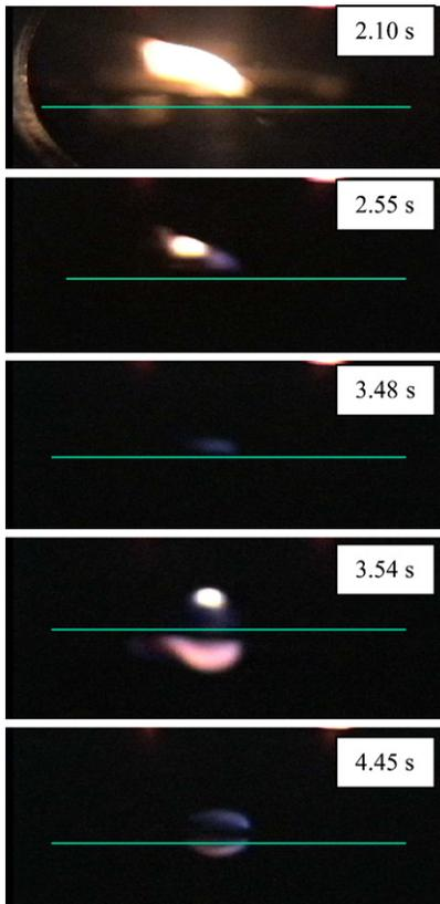
Fig. 2. Selected edge view video images of flame behavior over 0.2 mm thick PMMA sheet (green line) in 21% O<sub>2</sub> at 5 cm/s flow from right to left. Laser irradiation from top.
