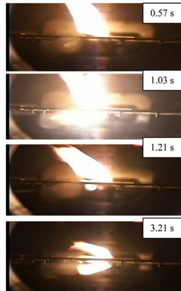
Fig. 4. Selected edge view video images of flame behavior over 0.2 mm thick PMMA sheet in 35% O<sub>2</sub> at 5 cm/s flow from right to left. Laser irradiation from top.
