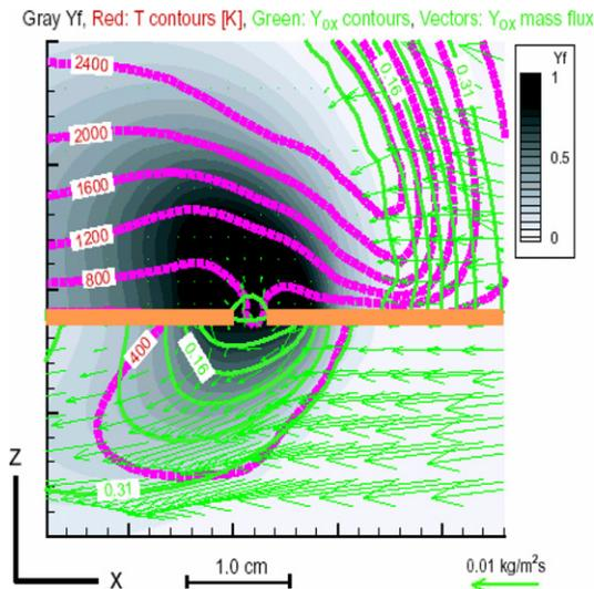
Fig. 7. Enlarged image of contours of fuel mass fraction, gas phase temperature, oxygen mass fraction, and oxygen mass flux vectors near the open hole over 0.2 mm thick PMMA with laser irradiation from top in 35%  $O_2$  at 5 cm/s flow from right to left at 0.64 s after the start of laser irradiation, shortly after a hole is formed in the fuel sheet.
