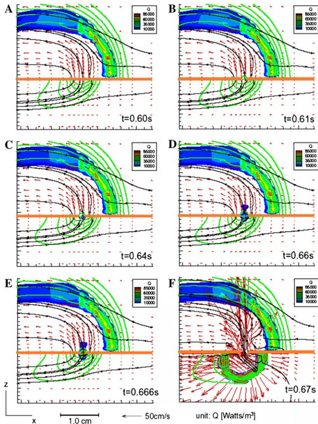
Fig. 6. Calculated two-dimensionally sliced contours, along the centerline, of heat release rate ( $Q$ ), oxygen mass fraction (green), stream line (black), flow vectors (red arrows) over 0.2 mm thick PMMA (orange sheet) with laser irradiation from top in 35%  $O_2$  at flow velocity of 5 cm/s from right to left at various times from the start of laser irradiation.
