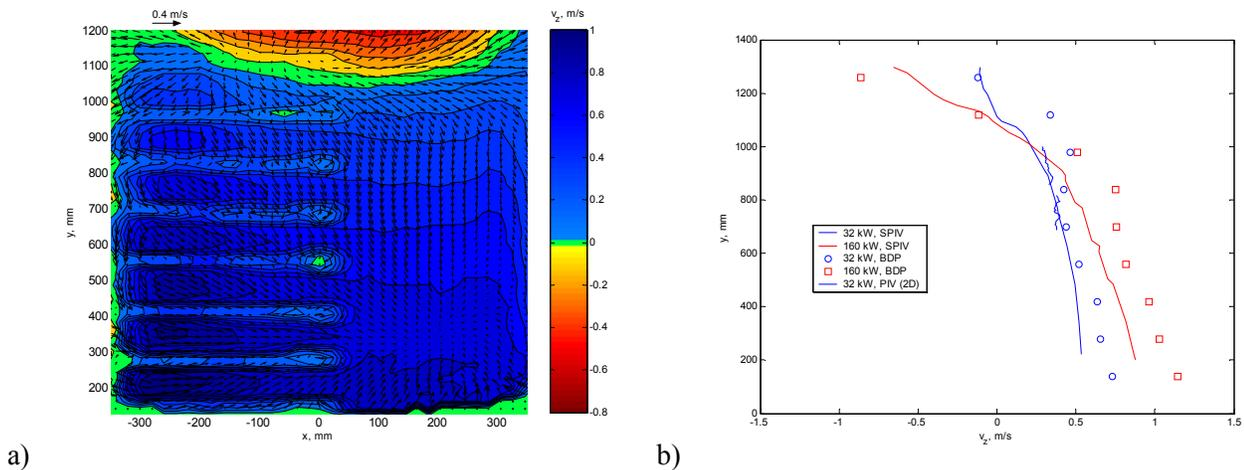
**Figure 1 a) Velocity vector field for the 160 kW fire. b) Comparison of centerline profiles of measurements from bi-directional probes, Stereoscopic PIV (SPIV), and traditional PIV (2D).**
