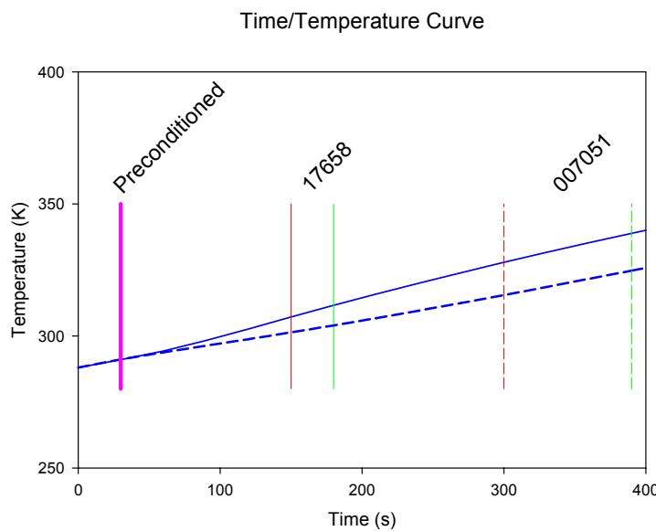
The figure shows the time/temperature curves for two of the scenarios used for testing the neural network. The numbers are sequence numbers of the scenarios (in this case from 1 to 20768). The green bars show the results of current detection strategies (set point and rate of rise). The red markers are the time for detection by the neural network, and the “preconditioned” marker shows the reduction in time after training with prior knowledge.
