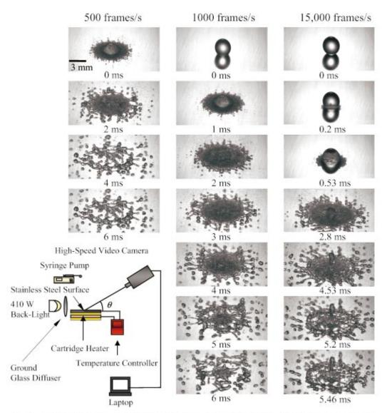
Droplet Impact on a Heated Stainless Steel Surface: Influence of Camera Framing Rate
