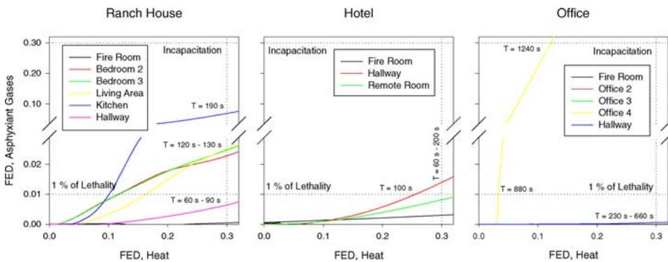
**Figure 4. Comparison of thermal effects and narcotic gas effects for several different geometries.**
